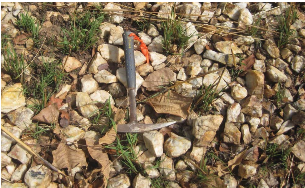
Figure 7-22: Pyrite-bearing quartz vein fragments on a dump (3.44 g/t Au)
