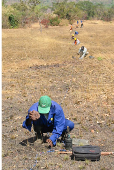
Example of ground Induced Polarization (IP) survey
